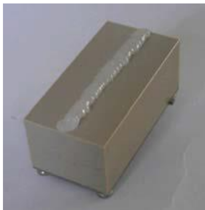
Figure 10 Application du couplant ultrasonique
